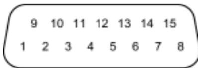
**Figure 23: Data Port Pin Layout**
