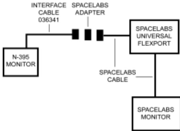
**Figure 21: SpaceLabs Connection**
